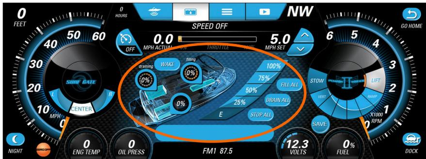
To **STOP ANY PUMP**, touch the tank indicator then touch **STOP**.
