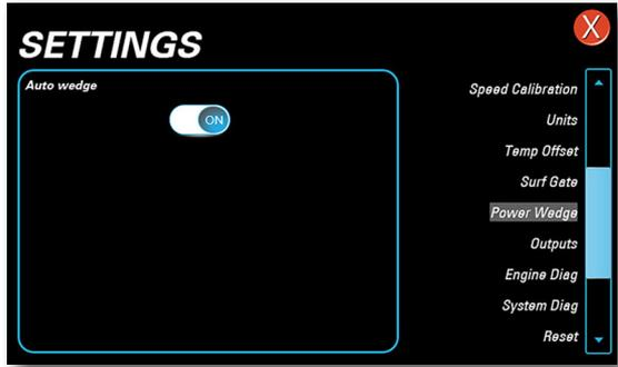
Touch **OUTPUTS** to **ENABLE/DISABLE** on-screen touch control buttons for optional equipment. When enabled, the buttons will appear on the screen.
