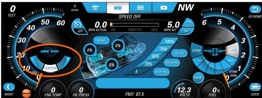
Surf **LEFT** or **RIGHT**, and **SWITCH** the wake from side-to-side with the touch of a Surf Gate control button. The selected position changes to **WHITE** and a progress meter appears until the position is achieved while the boat speed is 7.0 to 13.6 mph, and no alarms are active.
