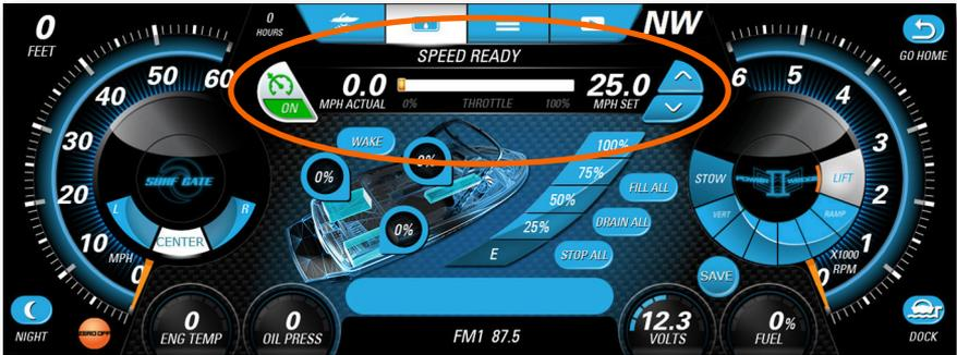
1. With the ENGINE RUNNING and in NEUTRAL, turn SPEED CONTROL ON by touching **SPEED CONTROL** button. The button will turn GREEN and ON will be displayed. "SPEED READY" is displayed above the THROTTLE BAR. Touching the speed control button again turns speed control OFF.
