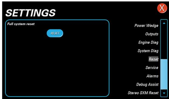
Touch **SERVICE** to view maintenance schedules recommended by the engine manufacturer. **SERVICE** notices will appear at each key cycle when the service hour interval has been reached, and must be cleared by the user.
