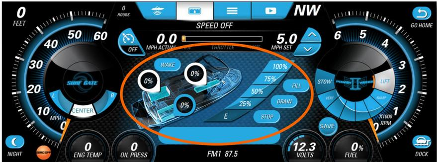
Tank indicators ALWAYS DISPLAY THE ACTUAL LEVEL IN THE TANK whether resting, filling or draining. Optional BALLAST BAGS can only be filled or drained by touching the **FILL ALL** or **DRAIN ALL** buttons.
