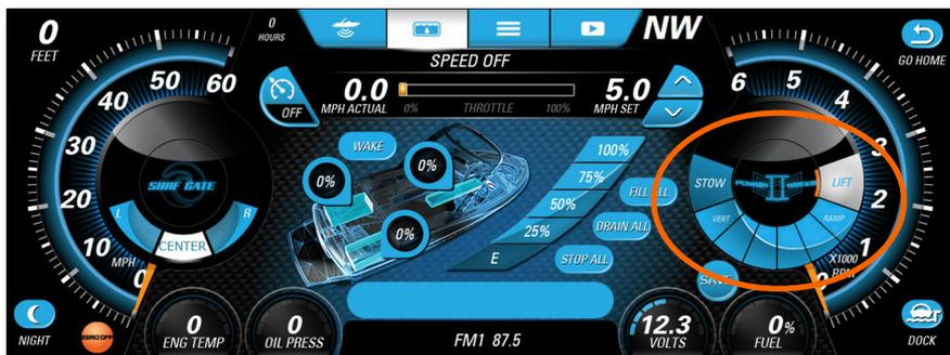
Before the ride begins DEPLOY the Power Wedge to a DOWNWARD position by touching any one of the 8 POSITION BUTTONS on the Power Wedge Control. If the wedge is in the STOW position (all the way up) you can press any of the remaining piano keys to DEPLOY the wedge.
