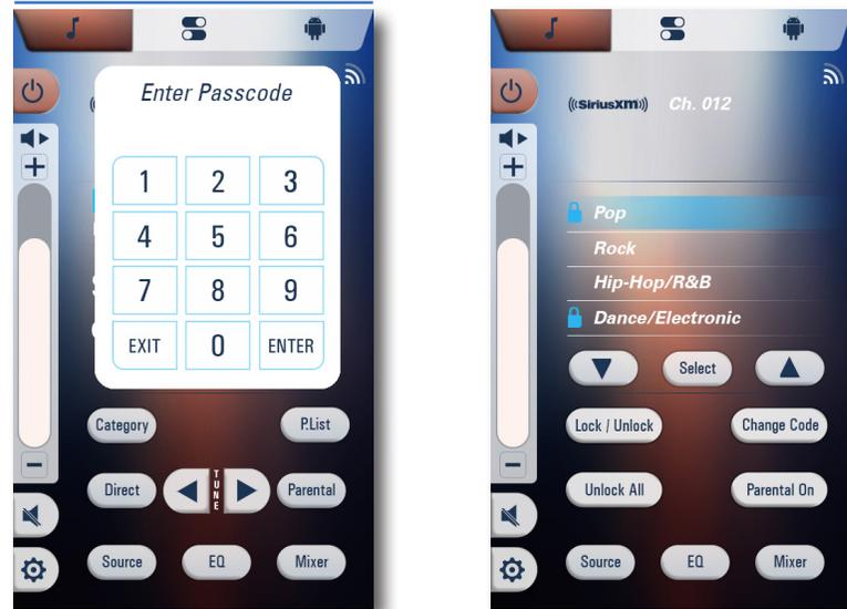
Limit the access to any SiriusXM Satellite Radio channel, including those with mature content. When enabled, the PARENTAL CONTROL feature requires a PASSCODE to tune to LOCKED channels. LOCKED channel information is not displayed without first entering a PASSCODE.
